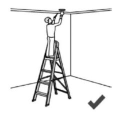
Use the right ladder for the job. For example, ensure the ladder is high enough for you to reach your work area without having to stand on the top rung.
