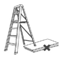
Place the ladder on stable and level ground. DO NOT place it on an uneven surface.
